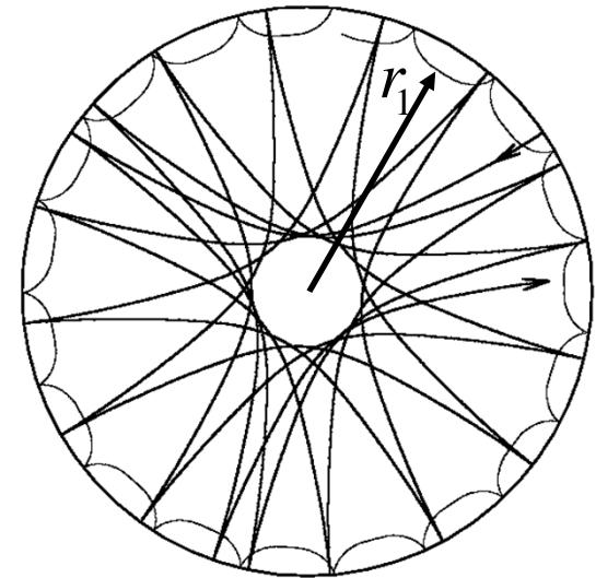
This equation has a simple physical interpretation:  $T$  is the travel time of acoustic waves to travel along the p-mode ray path; the right-hand side integral is an average of the sound-speed perturbations along this ray path.
