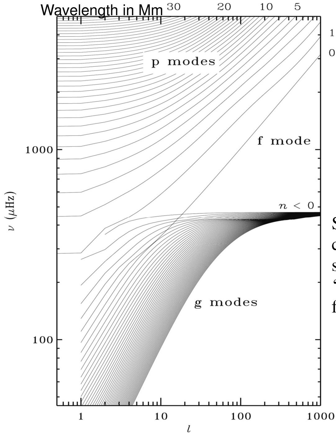
Spectrum of normal modes calculated for a standard solar model. Note the ‘avoided crossing effect’ for f and g-modes.
