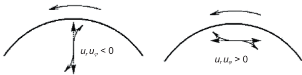
Figure 6 A sketch illustrating angular momentum transport in the equatorial plane by turbulent mixing. The direction of rotation is indicated at the tops. The left and right panels indicate how radially moving and horizontally moving fluid blobs are deflected by the Coriolis force. From Kitchatinov [44]. Note that Kitchatinov [44] has used u for the velocity of the blob, whereas we are using v .
